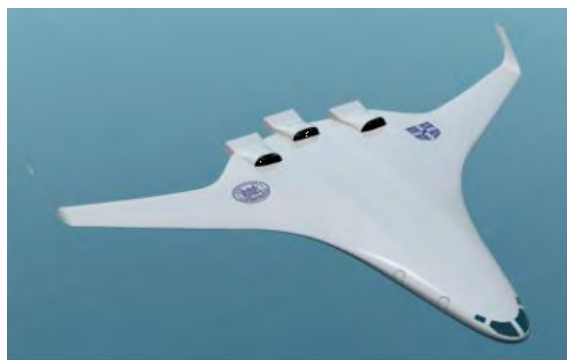
Figure 18: The 'Silent' Aircraft or blended-wing-body aircraft
