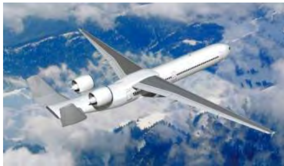
Figure 17: Study single-aisle aircraft demonstrating engine noise shielding by fuselage and tail plane
